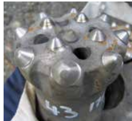
Norrtälje, Sweden. Secoroc Powerbit T45, 76 mm retrac, with HD Trubbnos buttons. The Trubbnos profile is re-created after grinding, keeping a wear flat area of about 10 %.
